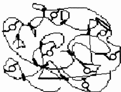
Figure 3. Scheme of the PZI hydrogel with chemical (○, EGDM bridges) and physical (■, ZC) junction points.
